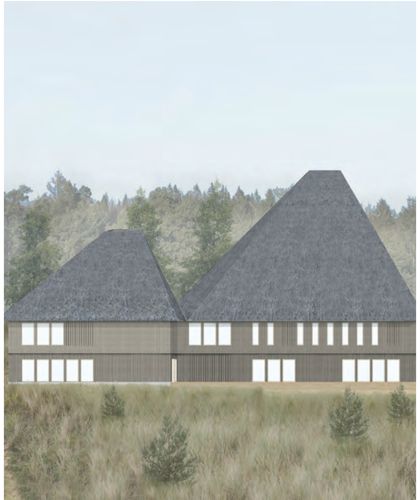
An elevation of the south façade: The façade is divided in two horizontal parts, with different wood cladding profiles, and wooden slats to create balance between the two levels.
