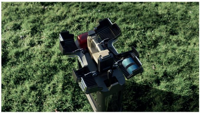
The mechanical opening presents both gun and tool for cleaning by the push of the handle.
