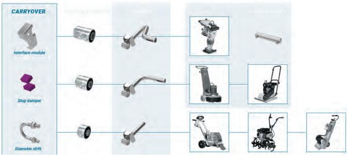
Vibrashifter is a system that is compatible with the machines presented. Every product for the machines includes the carryover components. The stop damper is available in different material stiffnesses.
