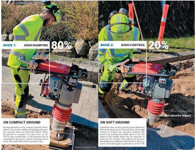
Vibrashifter solves the dilemma between efficiency and damping with MODE SHIFT. A feature that allows the operator to quickly adapt to the ever-changing conditions of tasks. The operator does not need to endure high vibration exposure when less control is needed.
